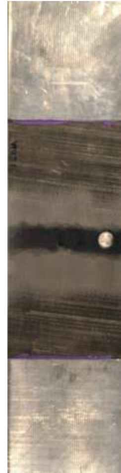
Fig. 4 Cold Expanded Specimen
